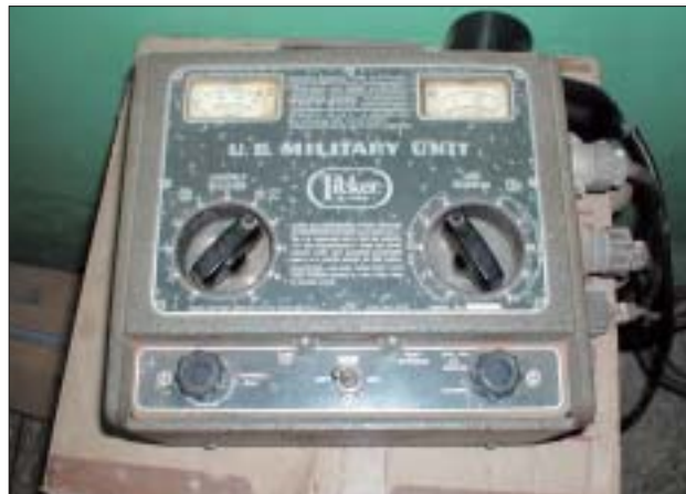
Figure 7: 1954 Picker control panel. Maximum output 15mA and 75kV.
